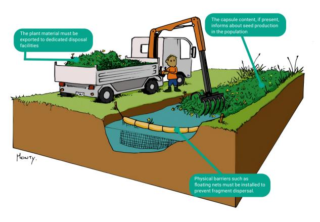
Fig 35. Mechanical removal of Ludwigia spp.
