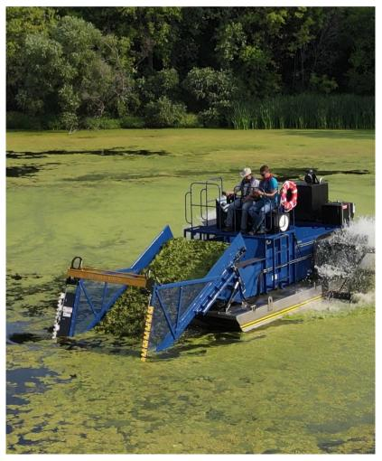
Fig 11. Mechanical removal using floating machines is ususally implemented in large water systems. Photo : Aquarius Systems
