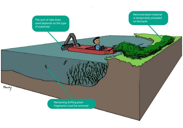
Fig 5. Mechanical removal of broadleaf watermilfoil using the harkboot
