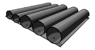
Fig 7. An example of an artificial refuge trap, consisting in pieces of PVC pipe riveted onto a metal plate and blocked on one side. It may be necessary to weight this type of trap with a stone, for example
