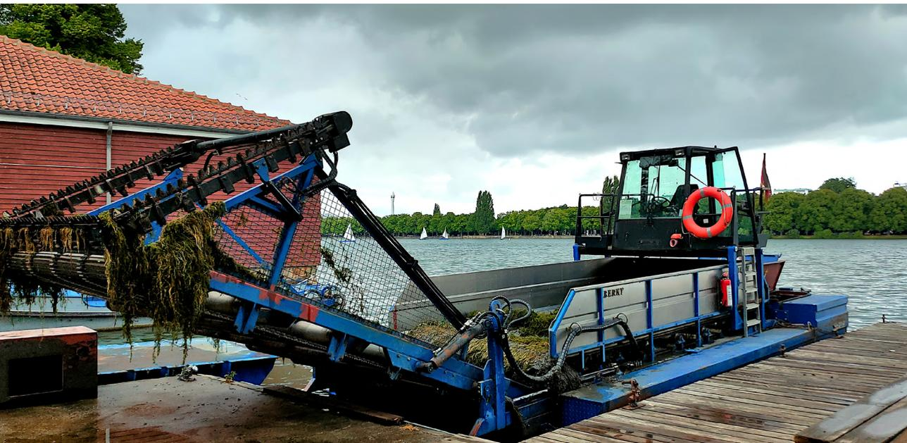
Fig 26. Example of aquatic weed harvester being used for the management of invasive aquatic plant species. Photo : Wassersalat
