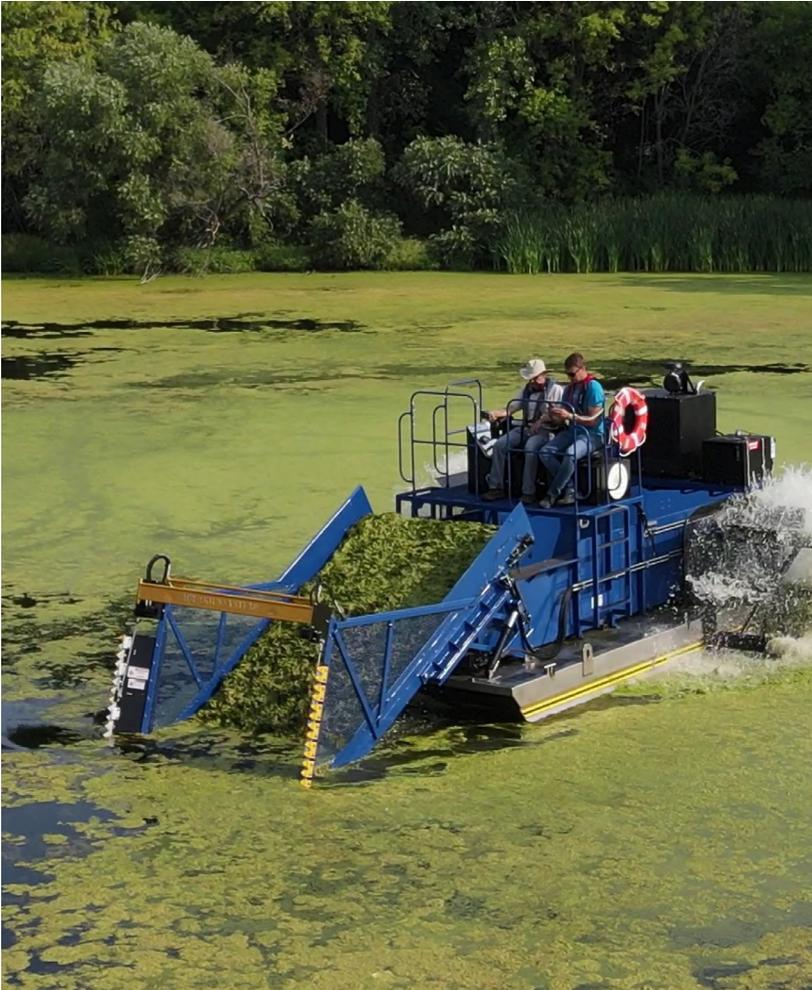
Fig 11. Mechanical removal using floating machines is usually implemented in large water systems. Photo : Aquarius Systems
