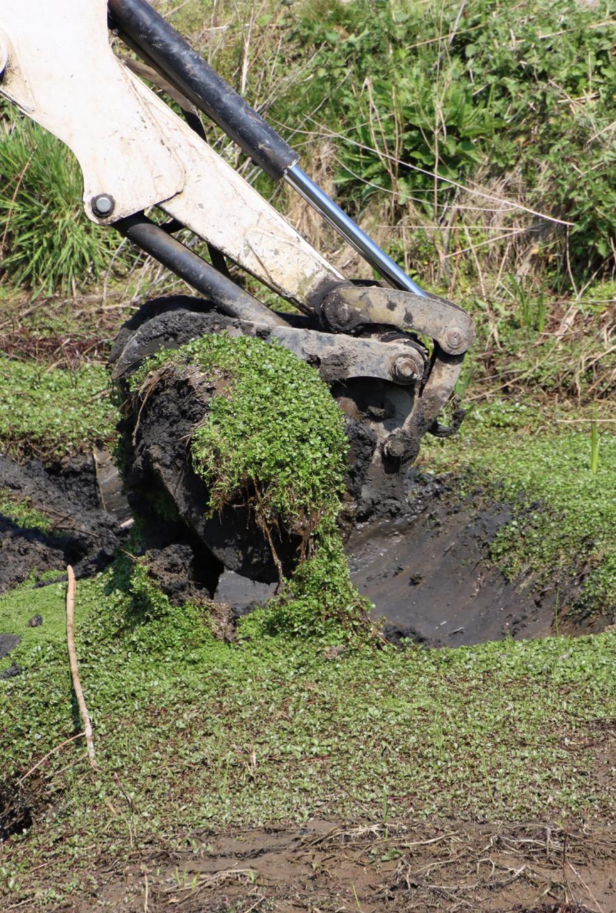
Fig 36. Mechanical dredging of water primrose after a complete drainage of the water body. Photo: Arnaud Monty
