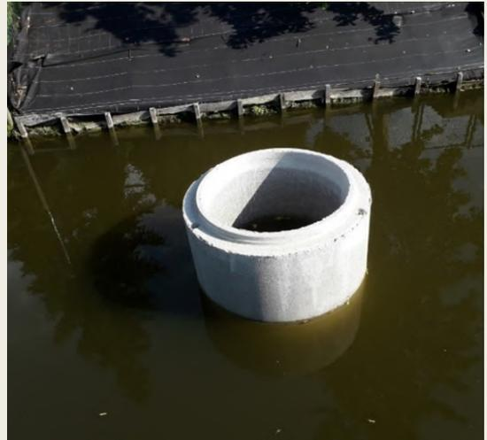
Fig 112. The concrete tube enabled operators to verify the effectiveness of the management without removing the fabric from the whole treated area. Photo: Provincie Oost-Vlaanderen dienst Integraal Waterbeleid
