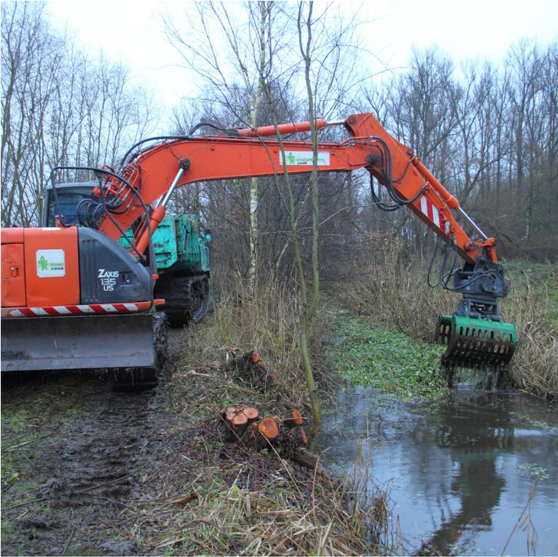
Fig 23. Excavators placed on the bank to remove floating pennywort from a narrow water system. Photo: Jérémie Guyon
