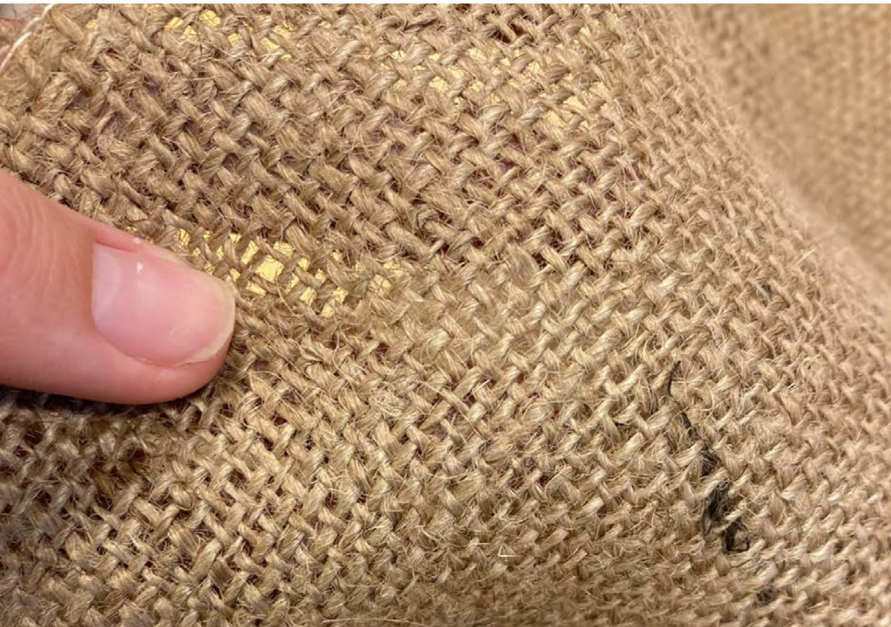
Fig 6. The fabric's holes must be small enough to prevent the plant from growing through the matting. Photo: Marie Patinet
