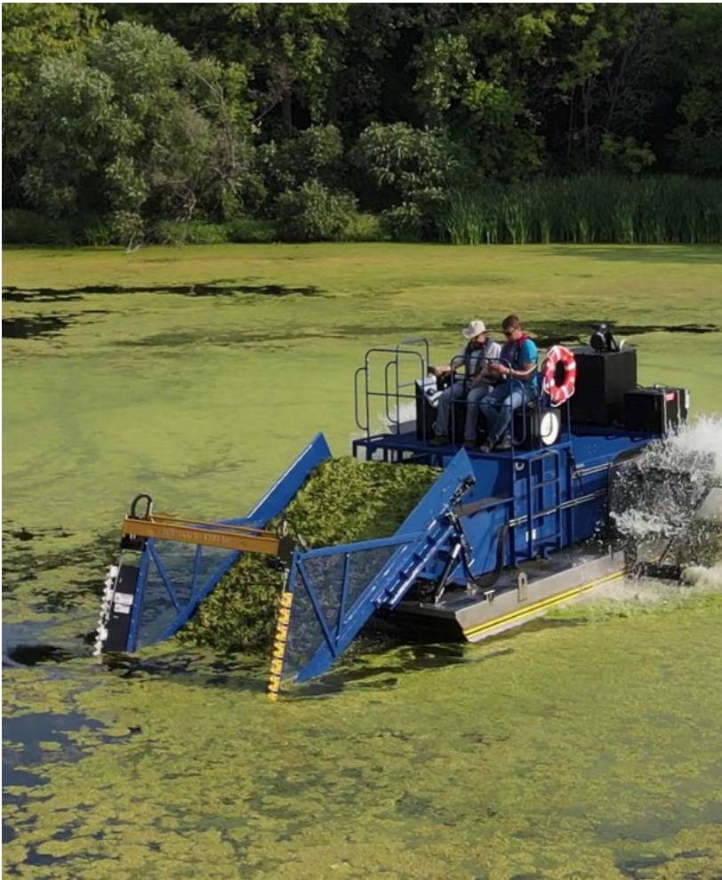
Fig 4. Mechanical removal using floating machines is usually implemented in large water systems. Photo : Aquarius Systems
