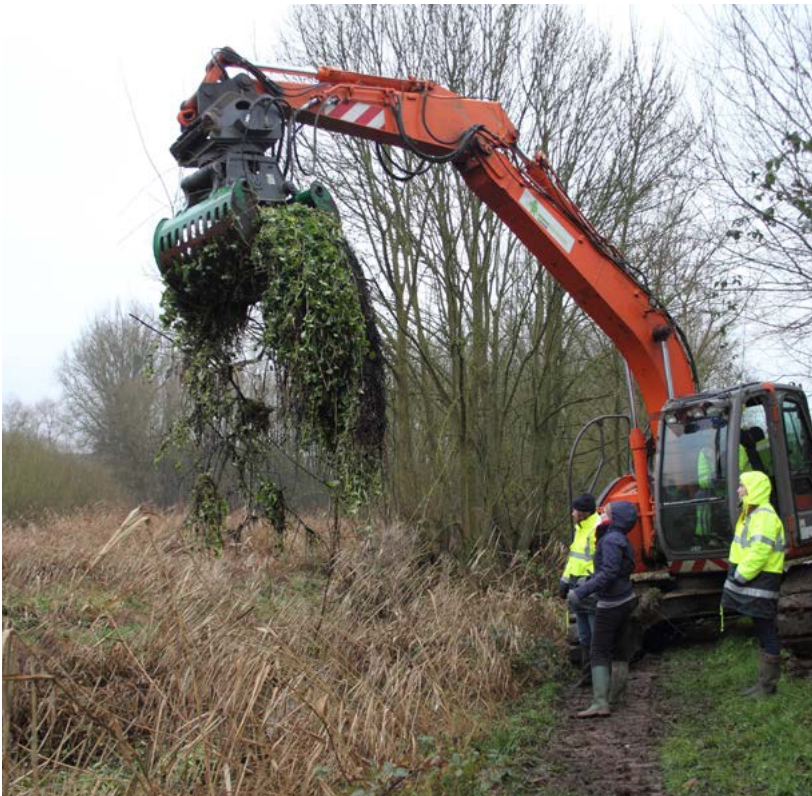
Fig 8. Excavators placed on the bank to remove floating pennywort from a narrow water system. Photo: Jérémie Guyon
